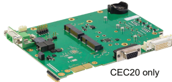
CEC20 only FIME mPCIe expansion DVI, VGA, 2x 2.5Gbit LAN
