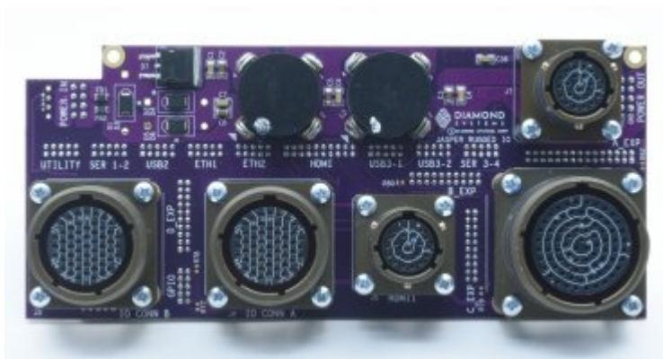
Panel I/O board eliminates most cables and provides built-in expansion capability
