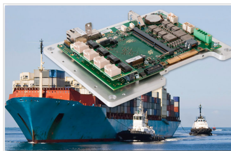
Open-Frame version, used in maritime environment with locking headers
