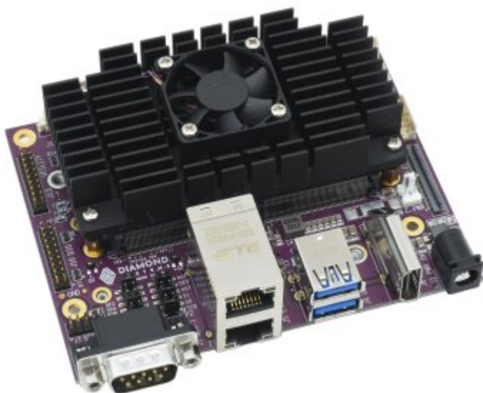
Jackson carrier with Orin NX and fan sink installed
