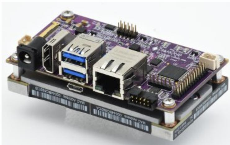
**Angle view with TX2 module installed underneath**
